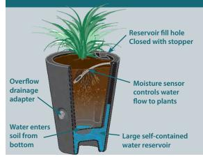
How Tournesol's Container Irrigation Works:
